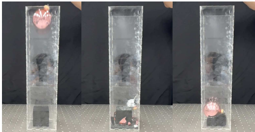
Fig. 22. Drop experiment with a glass Christmas ball with infill. The pictures before (left) and after the shock with a solid cube (middle) and optimized microstructure (right) at the bottom are shown.
