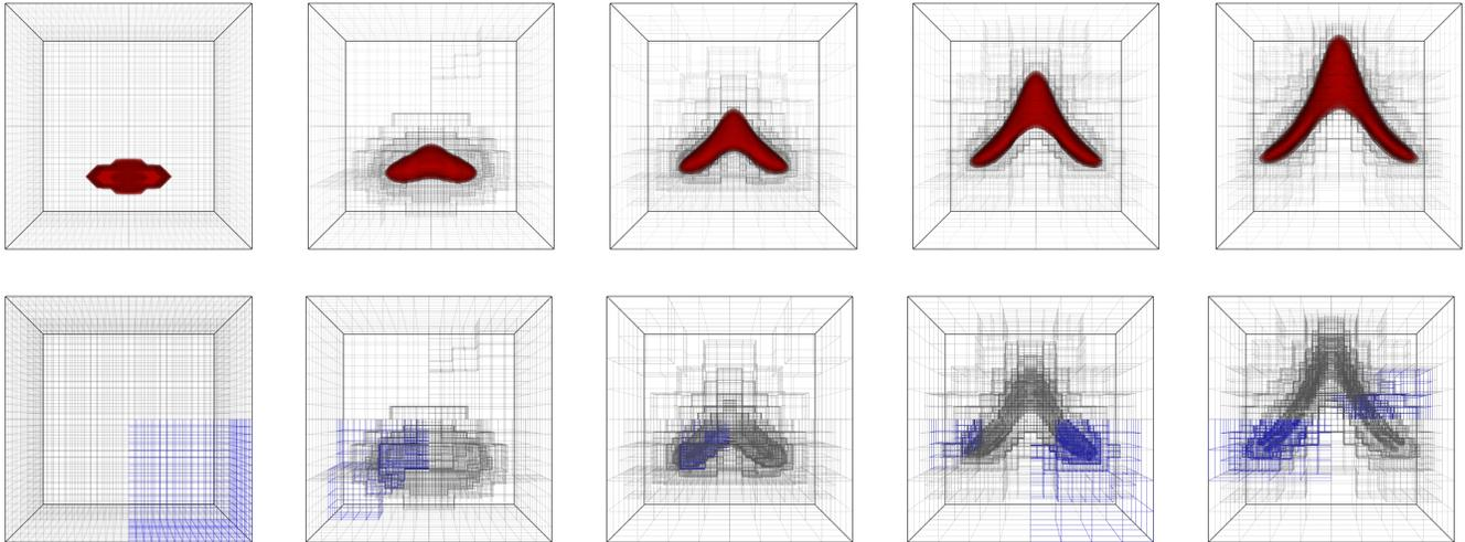
Figure 6: Illustration of mesh adaptivity for advection-diffusion equation (1) on 8 cores with a vertical flow field. The figure shows snapshots of isosurfaces of the transported quantity  $C$  at five time instants (upper row) and corresponding adapted meshes (lower row). The blue elements in the lower row belong to Core #3, indicating the dynamic evolution of the mesh partition.
