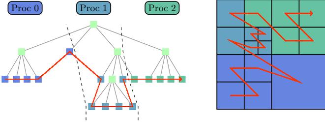
Figure 2: A pre-order traversal of the leaves of the octree in the sequence of triples  $(z, y, x)$  creates a space-filling curve in  $z$ -order. This imposes a total ordering of the mesh elements, also known as Morton ordering. A load-balanced partition of the octree is determined by partitioning the space-filling curve into segments of equal length. The globally shared information required for this operation amounts to one long integer per core.
