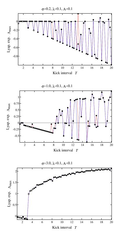
Figure 3: Effect of increasing shear on the Lyapunov exponents of the periodically-kicked linear shear flow. Note that  $\Lambda_{\max}$  is the rate of expansion per kick. Squares indicate that the corresponding  $F_T$ -orbits have veered outside the region |y| < 0.15; circles indicate that they have not. Upper and lower estimates of  $\Lambda_{\max}$  are both shown (see Simulation Details).
