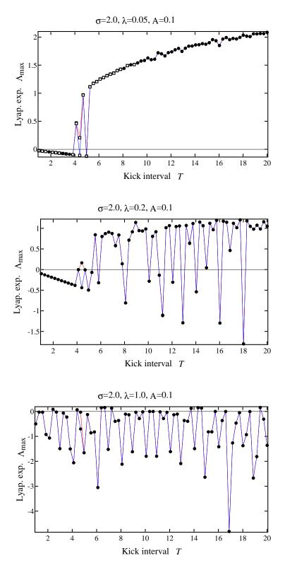
Figure 4: Effect of increasing damping on the Lyapunov exponents of the periodically-kicked linear shear flow. Squares indicate that the corresponding  $F_T$ -orbit has veered outside the region |y| < 0.15.
