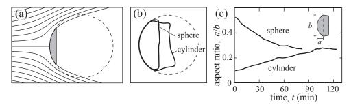
Figure 5: The terminal shape of a dissolving body. (a) 2D free-streamline theory predicts a shape of nearly constant curvature along its front. (b) Fitting a circle to the late-time experimental interfaces also reveals fronts of nearly constant curvature for initial shapes of a sphere and an axially-aligned cylinder. (c) Frontal aspect ratios of these two initial conditions converge to similar terminal values.
