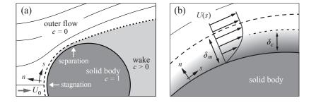
Figure 3: Schematics of the flow and concentration fields. (a) The steady outer flow consists of fresh water, while the attached flow near the body forms a boundary layer (dashed line) containing dissolved material. (b) Zoomed-in view of the momentum and concentration boundary layers (not to scale), the former defined by the flow velocity and the latter by the solute.
