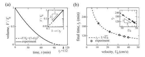
Figure 4: Scaling laws for dissolution in flow. (a) Decrease in volume over time for an initial sphere. Experimental measurements (solid curve) agree closely with the predicted power law (dashed curve). Inset: Logarithmic-scale plot of normalized volume and time. (b) Total time to vanish as a function of flow speed for experiments (dots) and theory (dashed line). Inset: Logarithmic-scale plot.
