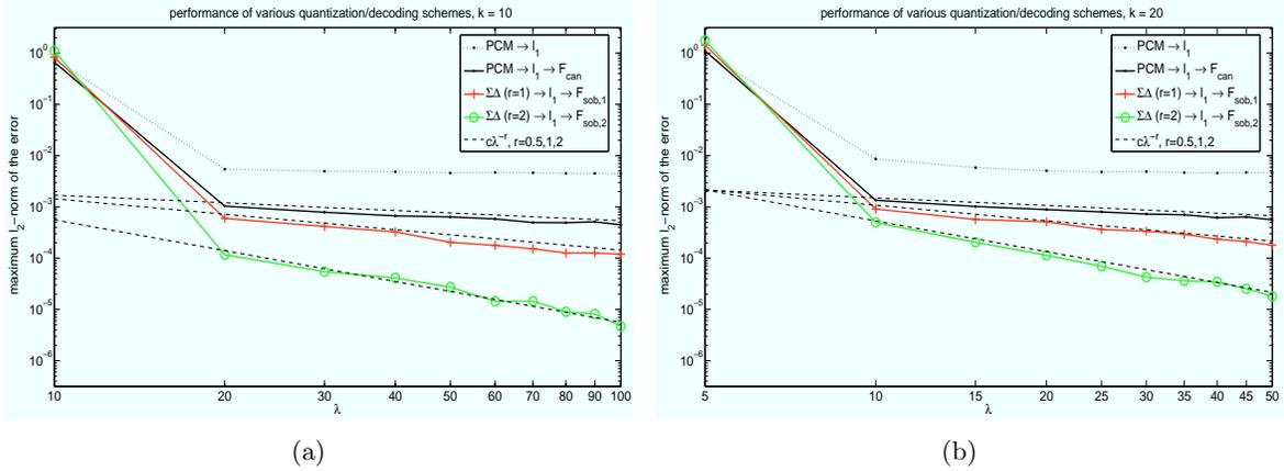
Figure 2: The worst case performance of the proposed  $\Sigma\Delta$  quantization and reconstruction schemes for  $k = 10$  and  $k = 20$ . For this experiment the non-zero entries of  $x$  are constant and  $\delta = 0.01$ .
