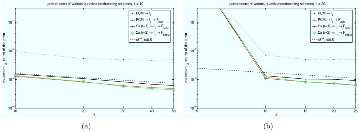
Figure 4: The worst case performance of the proposed  $\Sigma\Delta$  quantization and reconstruction schemes (with general duals) for  $k = 10$  and  $k = 20$ . For this experiment the non-zero entries of  $x$  are constant and  $\delta = 0.01$ .
