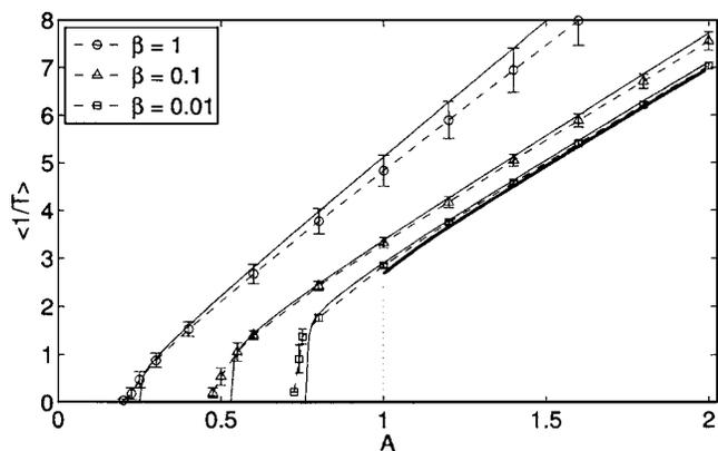
FIG. 4. Bifurcation diagram for the noise-induced limit cycle. Points are results of the simulations with  $\alpha = 10^{-5}$ , thin lines are theoretical predictions for the corresponding values of  $\beta$ . The thick line is the bifurcation diagram in the absence of the noise in the limit  $\alpha \rightarrow 0$ .
