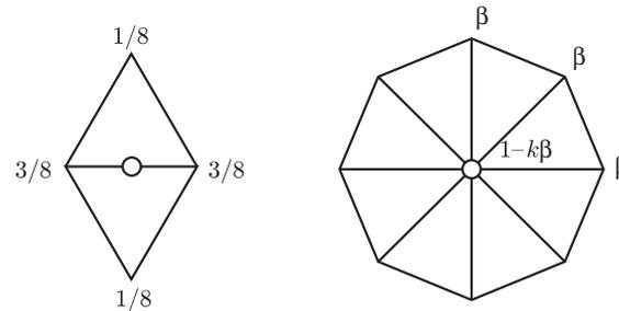
Fig. 3. Loop subdivision masks for new control points and updated positions of old control points. Vertices, for which control points are computed, are marked with circles.
