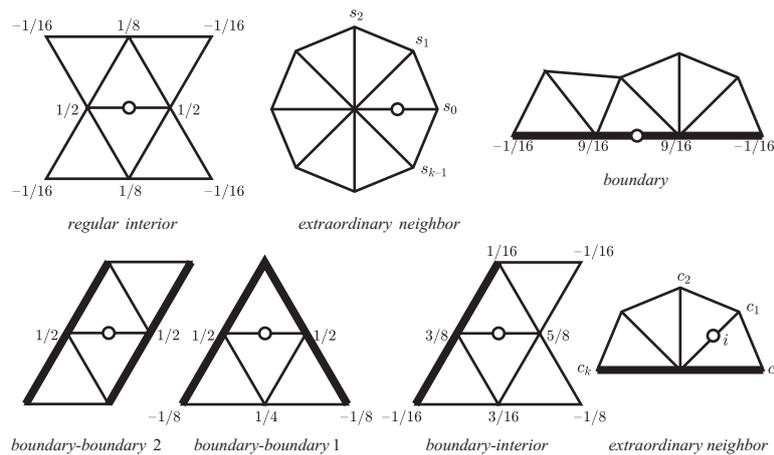
Fig. 7. Modified Butterfly subdivision. The coefficients  $s_i$  are  $\frac{1}{k} (\frac{1}{4} + \cos \frac{2i\pi}{k} + \frac{1}{2} \cos \frac{4i\pi}{k})$  for  $k > 5$ . For  $k = 3$ ,  $s_0 = \frac{5}{12}$ ,  $s_{1,2} = -\frac{1}{12}$ ; for  $k = 4$ ,  $s_0 = \frac{3}{8}$ ,  $s_2 = -\frac{1}{8}$ ,  $s_{1,3} = 0$ .
