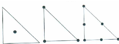
Fig. 8.8. Local interpolation nodes on \hat{T} for k=0 (left), k=1 (center), k=2 (right)
