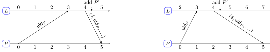
Fig. 6: The leader L 's clock running ahead (right) negatively affects liveness as the addition of P ' can be withheld longer from P .
