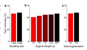
Figure 5: The effects of (a) frame rate, (b) segment length, and (c) data augmentation on classification accuracy in the downstream linear classification task with the labeled S dataset.
