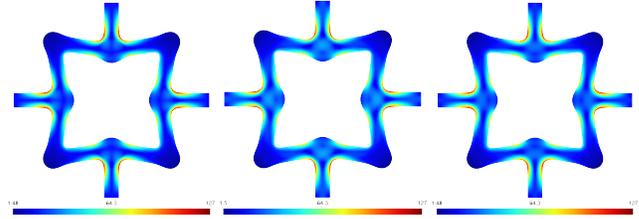
**Fig. 5.** The three worst-case microscopic stress measures from left to right: maximum principal stress, Frobenius norm, and von Mises stress. Each is efficient to compute exactly for every element in the mesh.
