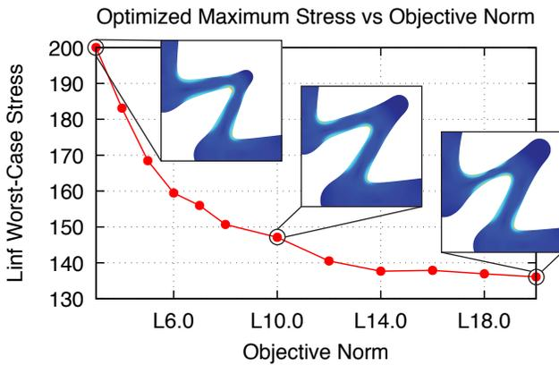
**Fig. 15.** The peak worst-case stress level and corresponding structures designed by minimizing the  $L_p$  worst-case stress norm.
