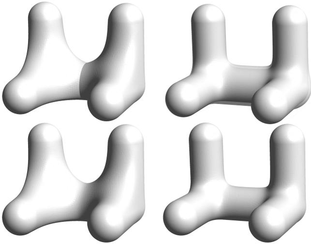
**Fig. 10.** *Top left: when two joints’ blending regions overlap, we must smoothly union them to avoid a sharp crease. Top right: blending using KS with spatially constant parameter  $s_{ab}$  dilates the shared edge even when no overlap exists, introducing bulging that violates printability. Blending with smoothing modulation  $\eta_F$  (bottom) solves both problems.*
