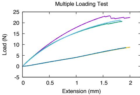
**Fig. 19.** We compressed one optimized and unoptimized structure at 0.5mm/s to 2mm. We then unloaded each structure and repeated the experiment twice. The optimized pattern traced out three overlapping lines at the bottom: its moduli were unchanged. The unoptimized structure broke on the first compression (top curve), causing weaker behavior on the two subsequent compressions.
