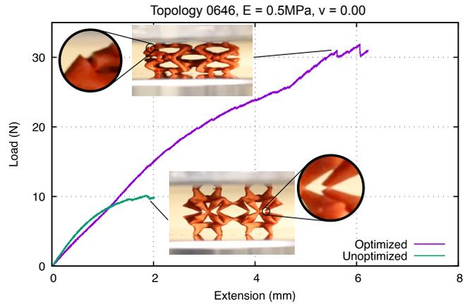
**Fig. 17.** We compressed unoptimized and optimized structures designed for the same material tensor until breakage. Despite the unoptimized pattern ending up slightly stiffer due to printing inaccuracies, it fails under much lower deformation.
