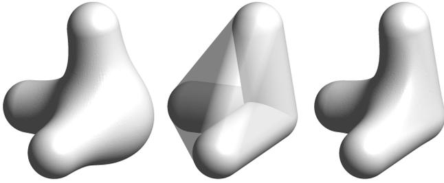
**Fig. 8.** *Bulging. Left: bulging exhibited by smoothed distance function; Center: blending region defined by convex hull; Right: smooth, bulge-free joint.*
