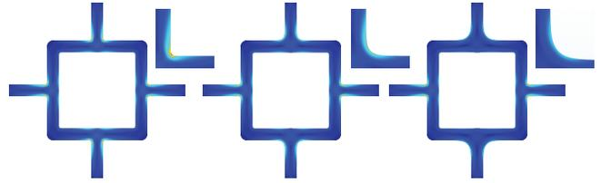
Fig. 2. The stress a microstructure experiences depends strongly on the structure’s corner smoothness.
