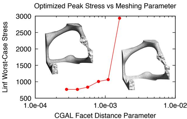
**Fig. 16.** Optimizations run at increasing mesh resolution from right to left (controlled by adjusting CGAL’s facet\_distance parameter to adaptively refine the surface mesh based on curvature), with the  $L_p$  norm of the stress of the final iterate evaluated on the fine mesh.
