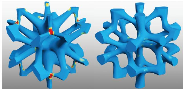
**Fig. 1.** We design microstructures emulating a desired material while simultaneously experiencing minimized peak stresses under the worst-case load. Here we show two structures with identical macroscopic properties. Our optimization smoothes out the stress concentrations seen in red on the left, creating a robust, organic microstructure. The meshes are shaded with our novel worst-case micro-stress measure.
