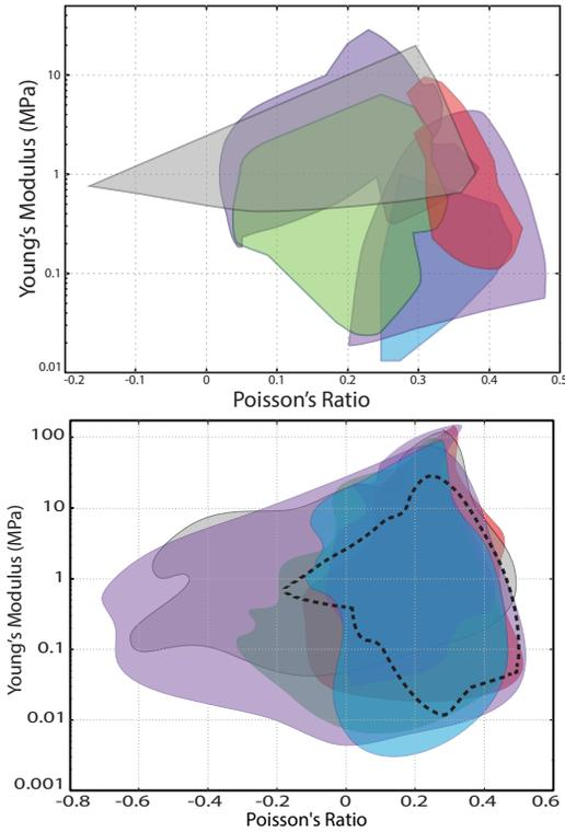
**Fig. 12.** Comparison of material properties covered by [Panetta et al. 2015] (top) and our optimization (bottom). Each colored region shows a single topology’s coverage, and the dashed curve at the bottom outlines the region from [Panetta et al. 2015].
