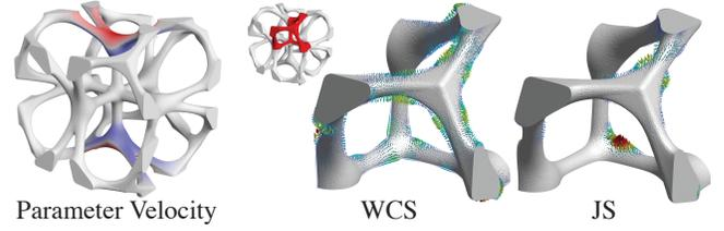
**Fig. 7.** Visualization of shape derivative quantities. Left: the normal velocity induced by changing a position variable, as computed by automatic differentiation of the signed distance function. On the right, the steepest descent velocity for our worst-case stress objective and the compliance tensor-fitting objective from [Panetta et al. 2015].
