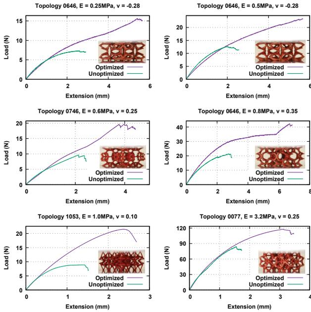
**Fig. 18.** Additional compression test results for a variety of topologies and material properties. A photo of the optimized pattern of each pair is inset. The optimized structure in the bottom left example did not actually break: it simply buckled into a lower energy configuration.
