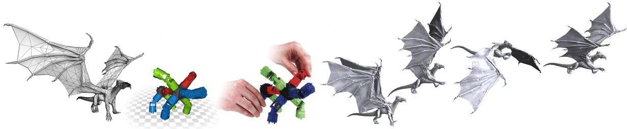
Figure 1: Left to right: Taking a rigged 3D character with many degrees of freedom as input, we propose a method to automatically compute assembly instructions for a modular tangible controller, consisting only of a small set of joints. A novel hardware joint parametrization provides a user-experience akin to inverse kinematics. After assembly the device is bound to the rig and enables animators to traverse a large space of poses via fluid manipulations. Here we control 110 bones in the dragon character with only 8 physical joints and 2 splitters. Detailed pose nuances are preserved by a real time pose interpolation strategy.
