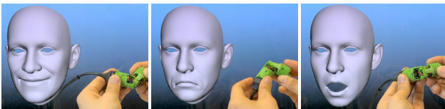
Figure 15: Controlling a face blendshape rig with a single joint. We manually map the angles of the joint such that they semantically match the facial expressions (i.e., a \vee shape for smiling, a \wedge for frowning, and twist opens the mouth).
