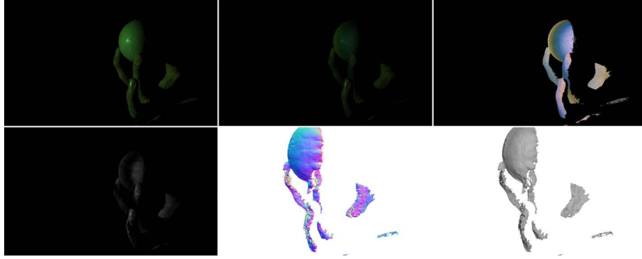
Fig.S57: Additional results: bouncy ball with Triton10 camera and analog projector. Top row: captured images from camera under uniform lighting and RGB pattern at 4.7ms exposure (both scaled \times 2 ), with the normalization \mathbf{I}_{\text{pattern}}/\mathbf{I}_{\text{white}} . Bottom row: fitted residual/ambient term (scaled \times 10 ), normals, and rendered 3D shape.
