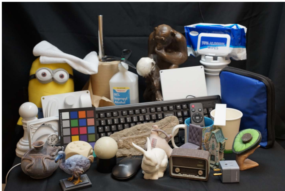
Fig. S6: Collection of Scanned Objects. We have scanned a collection of objects: from real-world, day-to-day items (keyboard, mug, alcohol wipes pack, cloth) to 3D printed objects (dodo, chair) to precisely milled ones (pawn, rook). This is to show the range of different geometries and materials that we can scan with NeLU3D .
