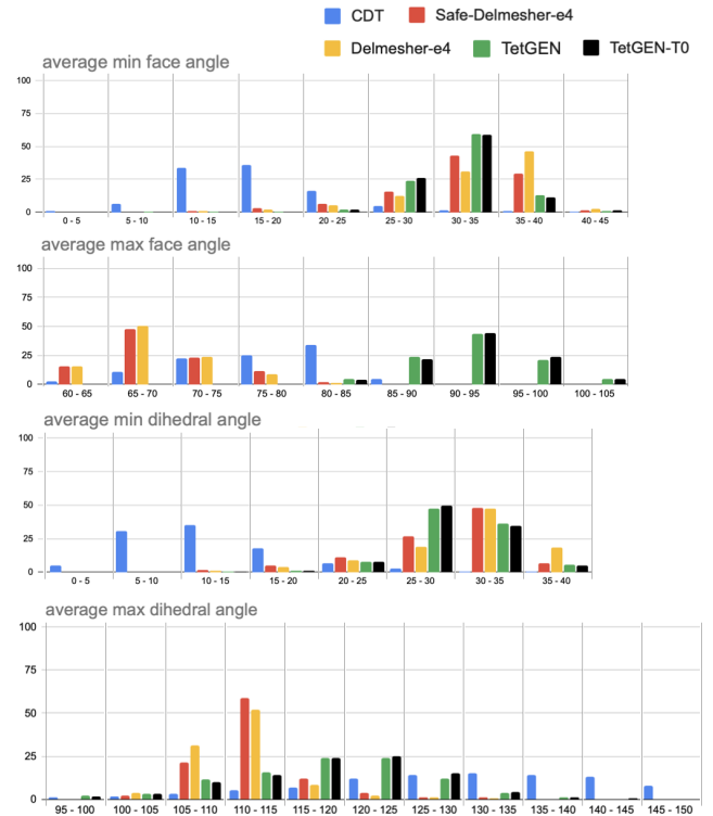
Fig. 11. Histograms showing the distributions of average angles among the meshes produced in our experiments. Here by average we consider an average-by-model . Specifically, the average min face angle of a given mesh is computed by summing the minimum angle of each face and then dividing by the total number of mesh faces. The same procedure involving maximum face angle is used to compute the average max face angle . Similarly, the average min/max dihedral angles of a given mesh are computed by summing the min/max dihedral angle of each tetrahedron and dividing by the number of tetrahedra. These histograms can be interpreted as in Fig. 10.
