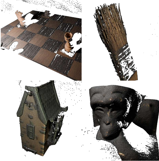
Fig. 5. Mosaic of Static Scenes with Ceiling Lights On. These static scenes were captured with our DLP Projector with ceiling lights on. Even though the lookup table was calibrated in a darkroom, LookUp3D is able to accurately reconstruct the objects. We show a chess board, a paint brush, a 3D-printed house, and a monkey statue, all reconstructed with 11 channels.
