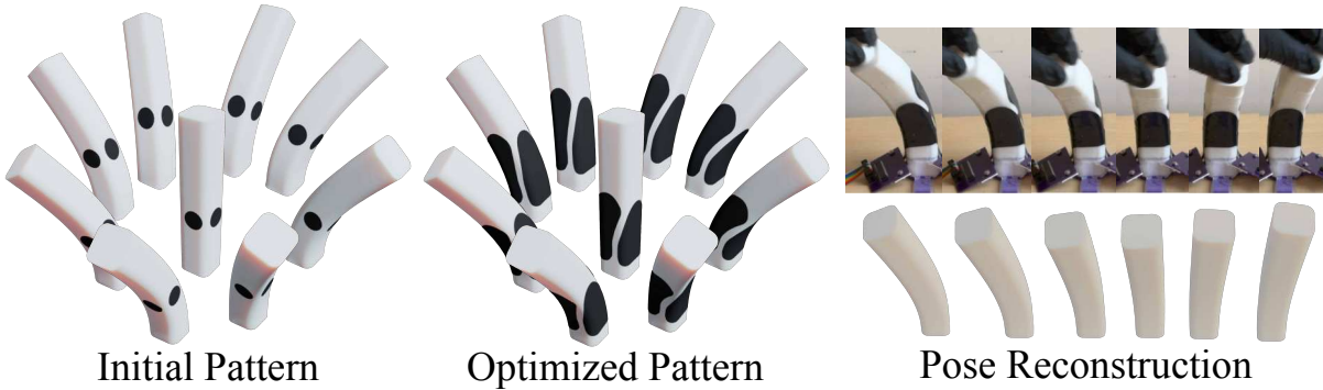
Fig. 1. Given a set of target poses, we find an optimal capacitive sensor array that maximally distinguishes between them. The sensor is fabricated using a silicone mixture and wrapped around the deformable object, providing major improvements when compared with a baseline, unoptimized sensor.
