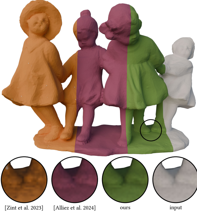
Fig. 36. Our method (green) is well suited for small offset distances. We use \delta = 0.01\% and set \ell_{\min} to the average input edge length (white) for ours and FPO (orange). For Alpha Wrapping (red), we set \alpha = 50\delta to achieve comparable edge lengths.
