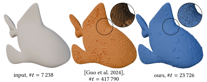
Fig. 5. Our method utilizes local subdivisions instead of a uniform refinement, leading to merely a fraction of triangles. Both, our method and [Guo et al. 2024], are guaranteed to construct an offset that is homeomorphic to a closed and manifold input mesh without self-intersections.
