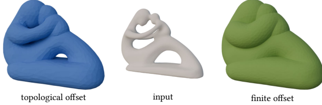
Fig. 3. Topological offsets (blue) always have the same topology for any given input (white), while the topology of finite offsets (green) depend on the offset distance
