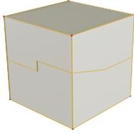
Fig. 2. An example of a feature configuration with no feasible solution. Aligned horizontal features in the middle of faces around the cube force all of them to have the same parametric coordinate (e.g., same  $u$ ). The vertical short feature line is labeled to be aligned with  $v$ , so can only have parametric length 0.
