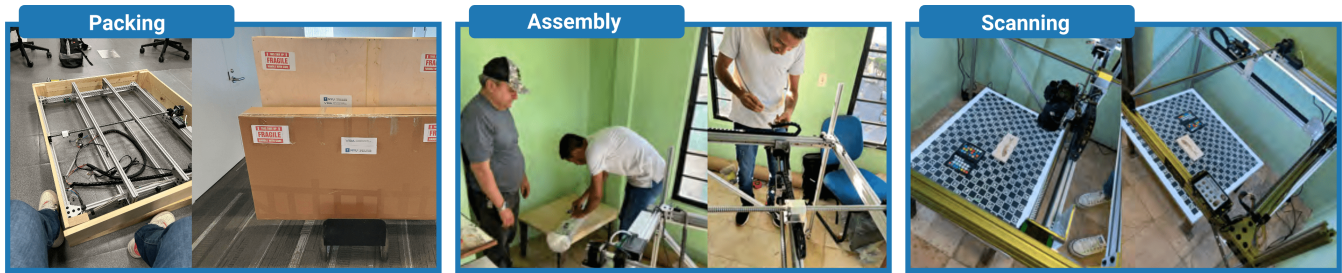
Figure 7: Deployment of the PaleoScanner required us to come up with a smart packing strategy that allowed us to safely carry the scanner to the field while enabling a streamlined reassembly process (See Section 6 for details). The PaleoScanner is currently deployed in the museum.
