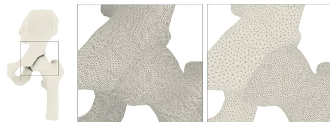
**Fig. 6.** The comparison between the surface mesh output from 3D Slicer and re-meshed surface mesh in fTetWild; The fTetWild result shows a clean mesh with no dense or erroneous triangles. The coarser mesh on the pelvic side guarantees robust contact definition in the FE analysis.
