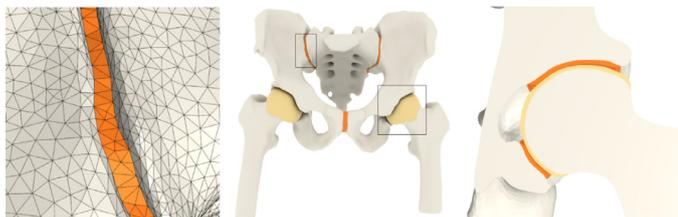
**Fig. 2.** The overview of our modeling features; Middle: the regions of interest cover the sacrum, the paired pelvic bones, the paired proximal femurs, and the three joints connecting these bones together; Left: all the bone-cartilage interfaces have conforming meshes. Right: congruent interfaces between the articular cartilages in the hip joint. (For interpretation of the references to color in this figure legend, the reader is referred to the web version of this article.)
