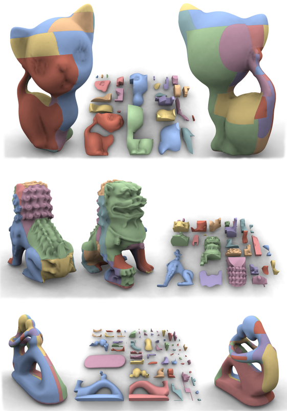
Fig. 13. Our method produces valid, compact decompositions for complex models containing: non-trivial topology (e.g., Fertility), thin features (e.g., the ears of the Kitten) and large portions not aligned with the global frame (e.g., the Chinese Lion’s body) for which manual decomposition is highly challenging to compute, resulting in 27 blocks for the Chinese Lion, 25 for Kitten and 63 for Fertility.
