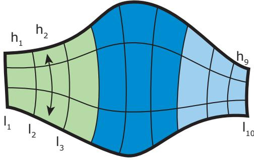
Fig. 1. We split strongly non-rectangular patches like this example patch by considering straight motorcyclines between two opposite sides of the patch having lengths  $l_i$  as cut candidates. We minimize isometric distortion by allowing power-of-2 multipliers between the segment heights  $h_i$ . A possible split is shown as colored segments.
