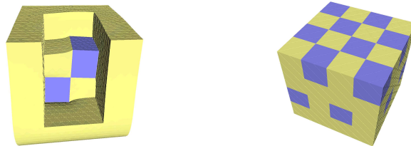
Fig. 1. Left: Two stiff cubic subdomains sharing an edge surrounded by softer material. Cubic domain \Omega cut open in front and on top.
