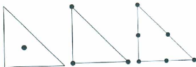
Fig. 8.8. Local interpolation nodes on \hat{T} for k=0 (left), k=1 (center), k=2 (right)
