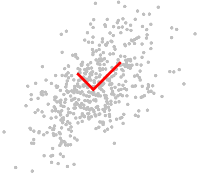
Figure 4: Samples from bivariate Gaussian random vectors with different covariance matrices are shown in gray. The eigenvectors of the covariance matrices are plotted in red. Each is scaled by the square root of the corresponding singular value s_1 or s_2 .
