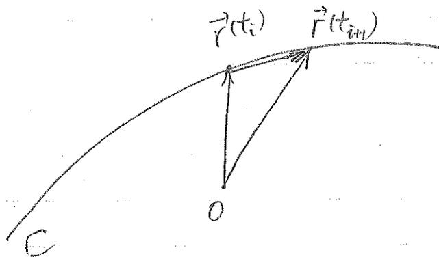
The spirit of this definition is the observation that when  $\vec{r}(t_i)$  and  $\vec{r}(t_{i+1})$  are close to each other,  $\vec{r}(t_{i+1}) - \vec{r}(t_i)$  is a good approximation of the curve between  $t = t_i$  and  $t = t_{i+1}$ .
