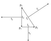
Figure 4: Vectors and points used in the membrane and bending strain calculations. The area of the triangle is A = (1/2)|n|.
