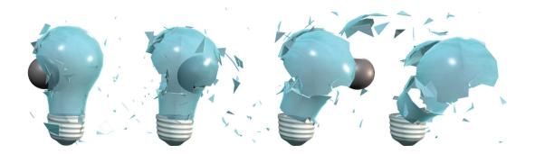
Figure 1: We used our novel measure of discrete strain to model plasticity and fracture of thin shelled objects. Shown are frames from our simulation of the shattering of a lightbulb.
