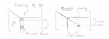
• Partial (row) pivoting permutes the rows (equations) of **A** in order to ensure sufficiently large pivots and thus numerical stability:
