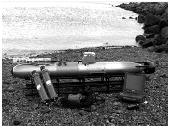
An autonomous underwater vehicle (AUV) and accessories of the type being employed by Prof. David Holland for his field research in Jakobshavn Fjord, Greenland.
