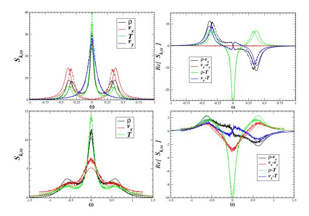
Figure 4: Diagonal (left) and the real part of the off-diagonal (right) components of the dynamic structure factor  $S_{k,\omega}$  for RK3D-2RNG (dashed lines) for the same parameters as in Fig. 3. For comparison, the analytical solution of the LLNS equations in Fourier space are also shown (solid lines). The imaginary part of the off-diagonal components is less than 0.1 and it vanishes in the theory. The top part shows the wavevector  $\mathbf{k} = (k_{max}/2, k_{max}/2, k_{max}/2)$ .
